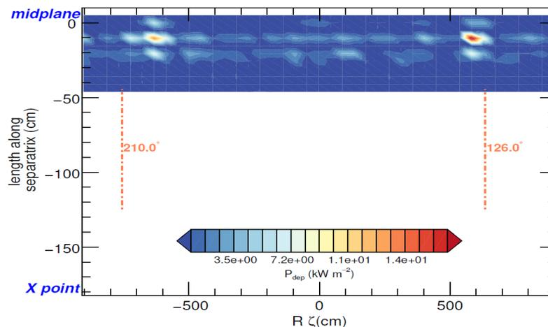
**Fig.2** Map of the power load (in kW/m<sup>2</sup>) calculated with a  $40 \times 10$  binning. In panel (b) the two vertical, dashed lines mark the injection and exit angles,  $\zeta_{inj} = 126^\circ$  and  $\zeta_{out} = 210^\circ$ .
