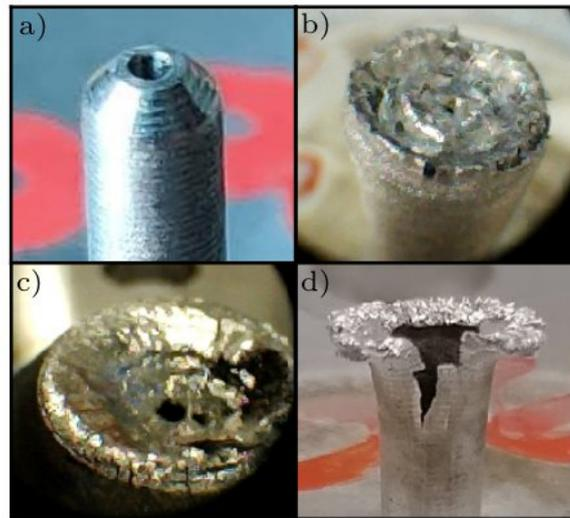
**Figure 1.** Gas jet nozzle damage observed on the Vulcan Petawatt laser by G. Hicks *et al.* [7]. (a) Nozzle prior to shot (b-d) Nozzles after a single full-power shot, with the laser focused 400  $\mu\text{m}$  above the nozzle tip. Extensive melting and cracking is observed.
