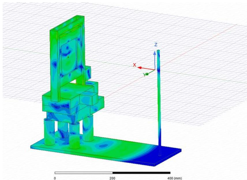
**Figure 1.** ELI MAIA target tower surface return current in 1.65 ns.
