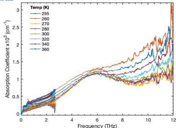
**Figure 2.** Water absorption coefficient as a function of temperature measured by broadband THz-TDS setup (continuous lines) and PCS THz-TDS setup (close circles).
