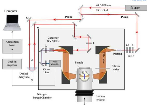
**Figure 1.** Broadband THz-TDS setup with THz pulse generation by two colors laser-induced air-plasma and ABCD technique.
