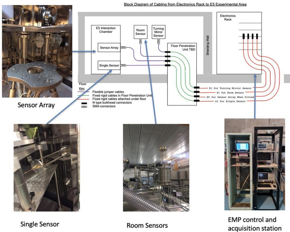
**Figure 1. Overview of EMP measurement system used in the commissioning experiments for particle acceleration with the 1 PW laser.**
