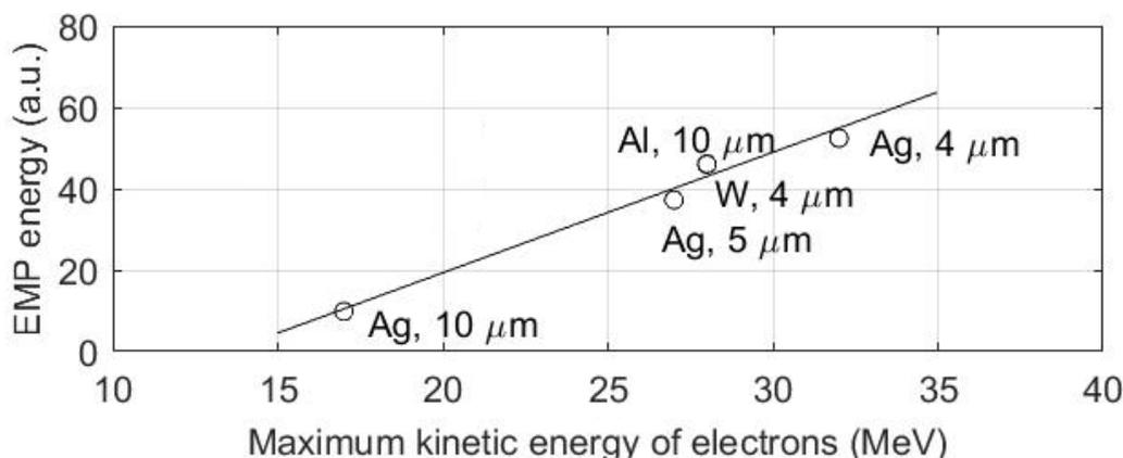
**Figure 1.** Electron maximal (recorded) energy from different material and thicknesses and produced EMP correlation
