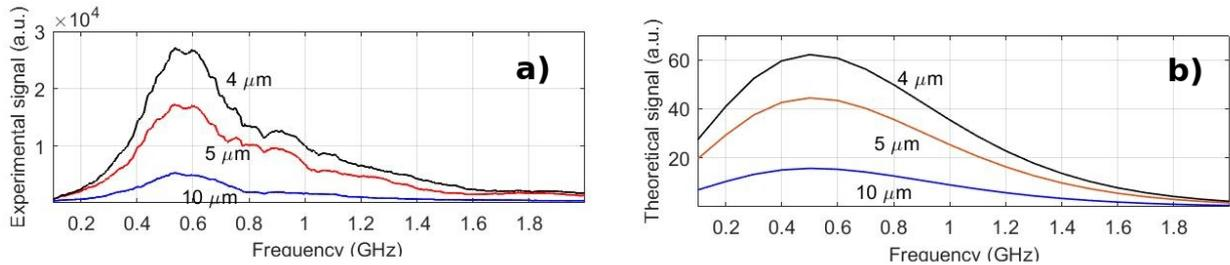
**Figure 2.** EMP generation in electron acceleration from Ag targets with different thicknesses
