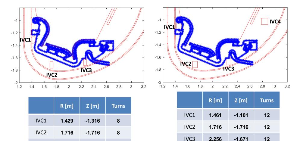
The limits adopted for currents and voltages on divertor coils are 5kA and 500V respectively
