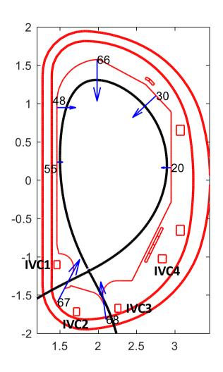
The sweeping control is a power exhaust strategy whose aim is to enlarge the divertor area affected by the plasma SOL imposing a periodic movement of the plasma divertor legs at a desired frequency with an almost fixed plasma shape.
