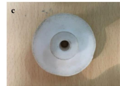
(a) Purging gas supply from downward to upward (b) Teflon cap of diameter 1 mm at top (c) Teflon cap of diameter 6 mm at bottom.
