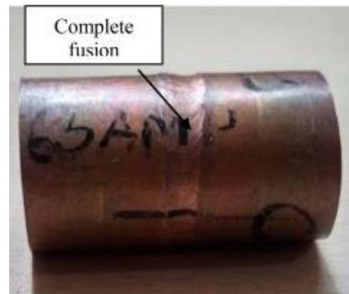
Orbital TIG welding of copper for high vacuum boundary applications [ https://doi.org/10.1016/j.ijpvp.2020.104225 ]
