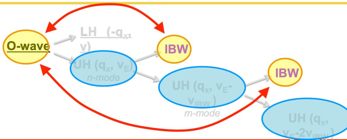
The **non-linear coupling of the daughter IBWs with the pump O-wave** can lead to the excitation of the **anomalous scattering** signal, down-shifted in frequency
