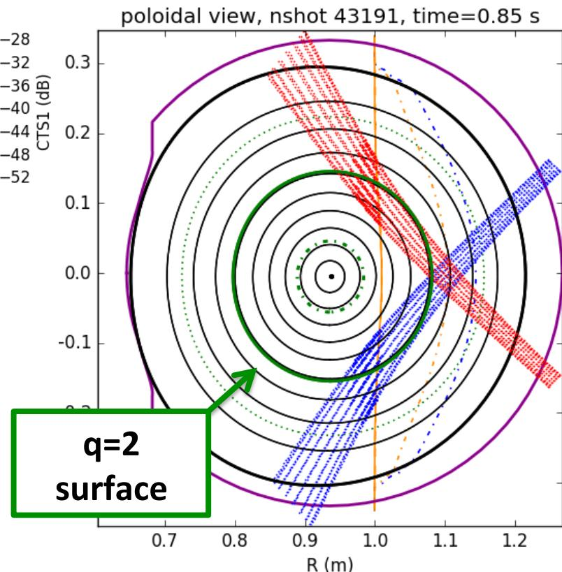
beams cross in an **outer** radial position wrt the **q=2** position
