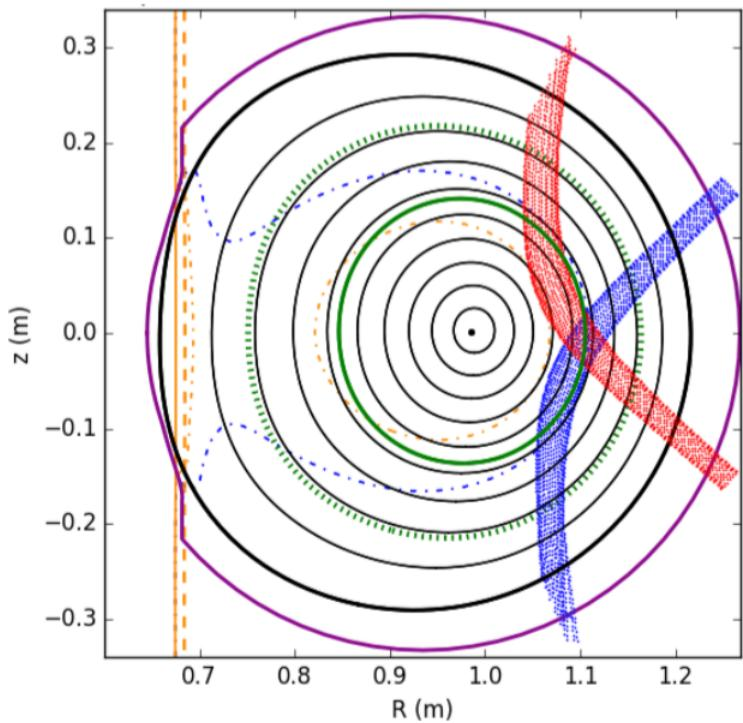
*Poloidal view of O-polarized beam launched (red) and received (blue) in the FTU shot #40282 at time 0.505 s. The  $q=2$  (3) rational surface is the green solid (dotted) line, the Upper Hybrid layer and X-mode right cut-off are the dash-dotted lines (yellow and blue respectively)*
