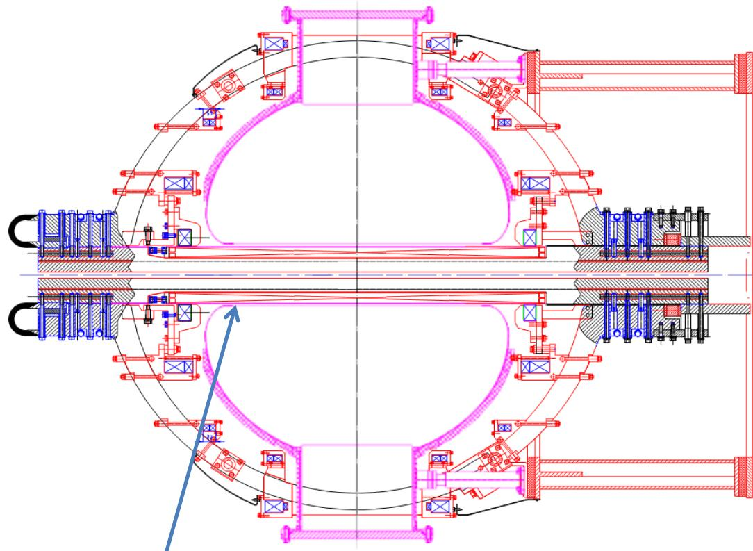
“Sliding layer” of 1mm separates Central Column from Central Solenoid
