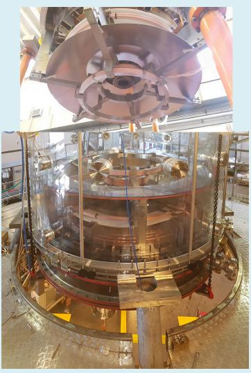
Confined plasma can be obtained without a nearby metal wall : the absence of any conducting shell distiguishes PROTO-SPHERA from any spheromak
