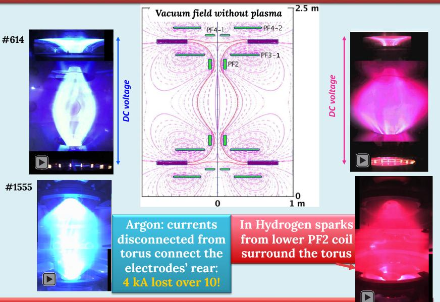
...but still in Phase-1.5 stray current paths are present around the tori ... curtailing the efficiency of helicity injection!
