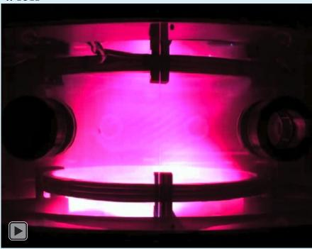
«Thin tori» (R/a=7, b/a=4) obtained in PMMA VV same as in 2018 Aluminium VV
