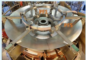
The 6 compression CPF coils fed by a Supercapacitor bank
