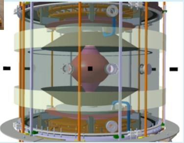
The presence of a gas blanket around the plasma cushions the inside of the 9 cm thick PMMA vessel
