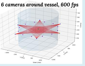
The transparent vessel allows for 3D plasma tomography in visible light
