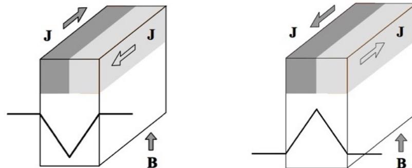
FIGURE 9. Screening currents induced by (a) rising and (b) falling field.
