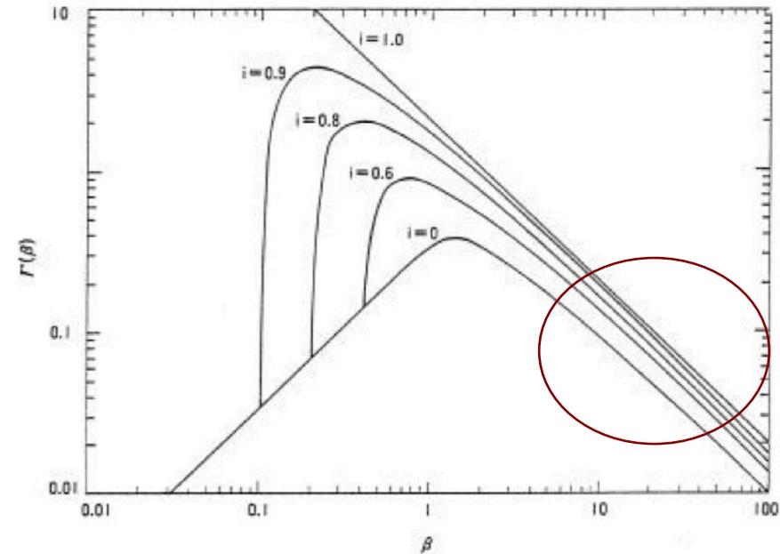
Figure 2.5: loss factor determining hysteresis losses for a slab carrying a transport current and subject to an external varying field.
