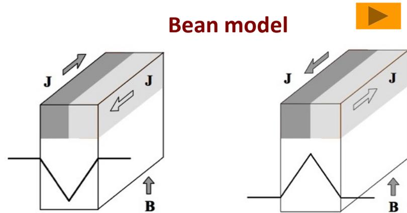
FIGURE 9. Screening currents induced by (a) rising and (b) falling field.
