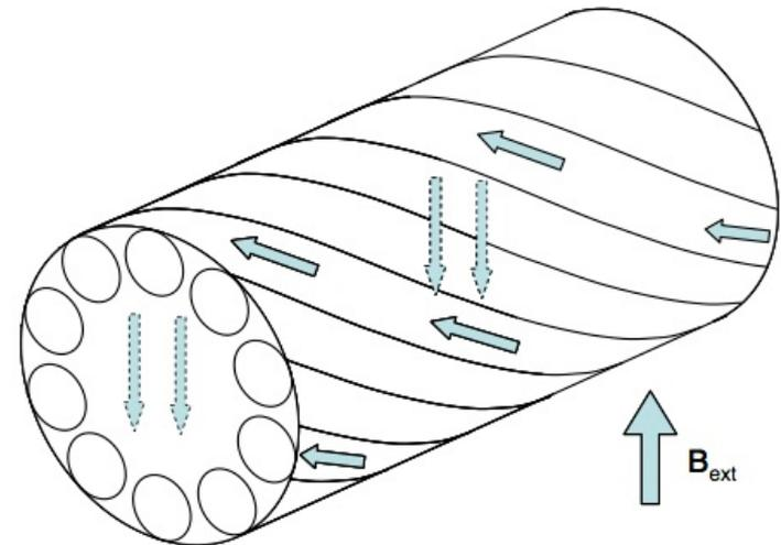
Fig. 2. The flow of coupling currents in a twisted composite wire.
