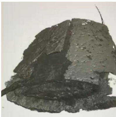
Fig.2: Volume rendering, obtained by X-ray tomography, of a portion of the sword shown in Fig. 1.
