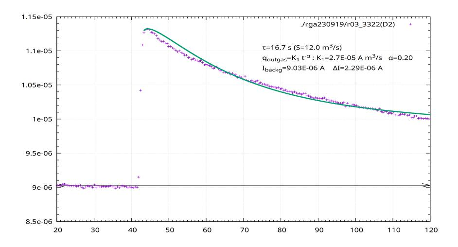
$au(RGA) \approx V_Q/S_Q \gg au_J(JET)$ ; outgassing high ( $\propto 1/t^{\alpha}$  with  $\alpha < 0.5$ ). Small sampling rate 2 RDGS/s (it is very difficult to resolve the initial transient).
