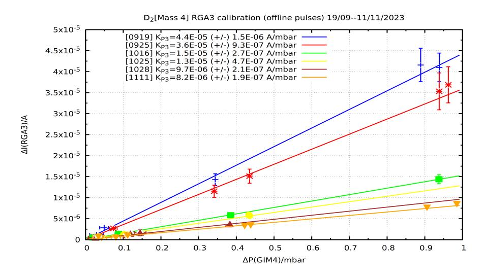
pumping conditions: torus sealed with T1 turbo pump, LN2 conditions, RGAs in SEM mode.
