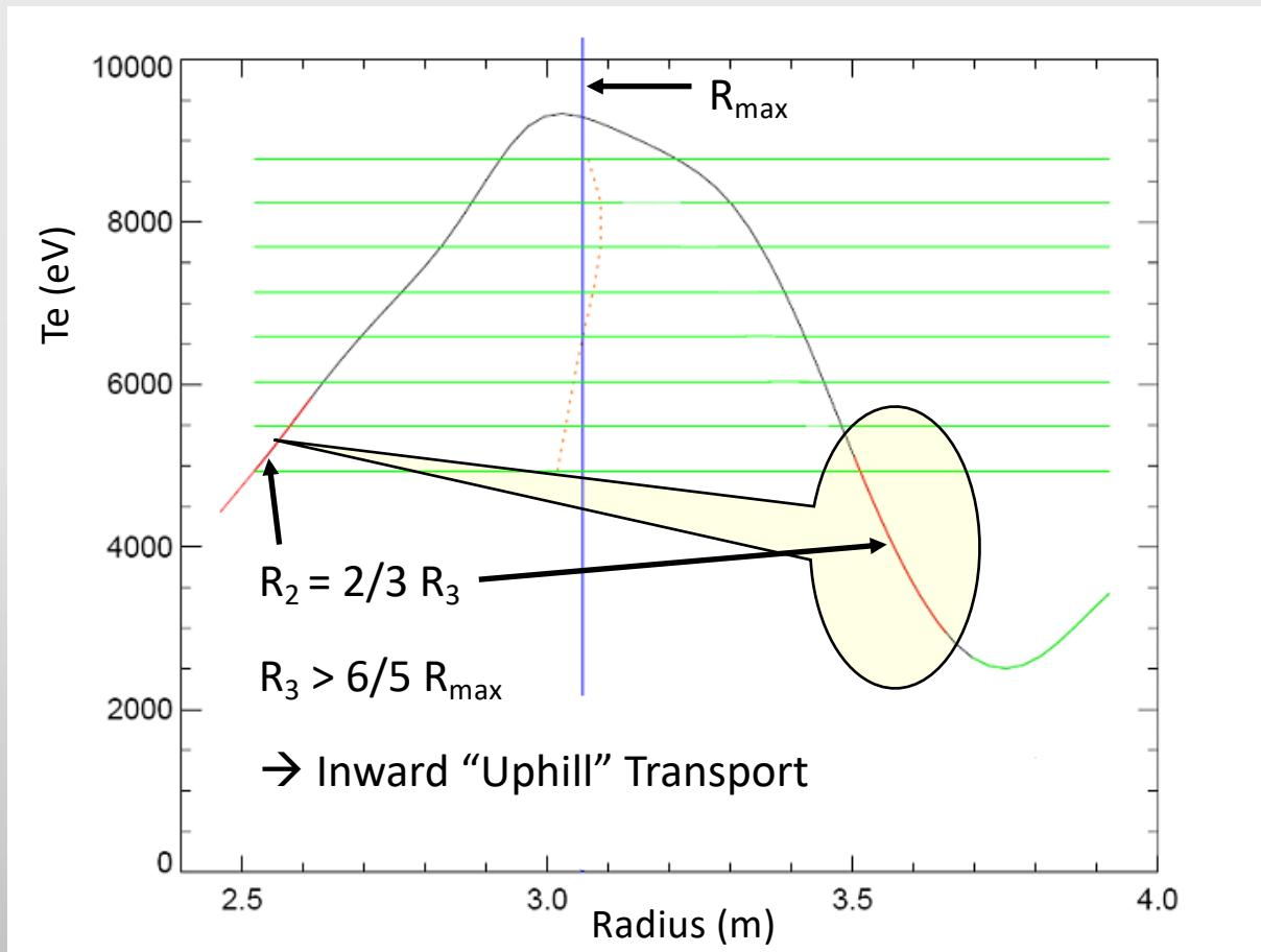
For high Te (>5 KeV) and high density, good ECE absorption coefficient and favourable transport conditions can enhance the inter-harmonic inward transport effect.
