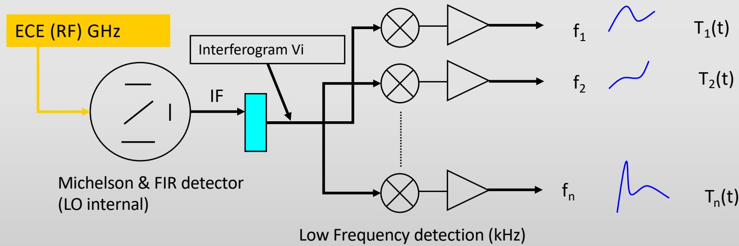
This method offers better time resolution of the traditional Fourier Transform analysis: a few wave cycles are sufficient to “clip” the ECE emission amplitude.
