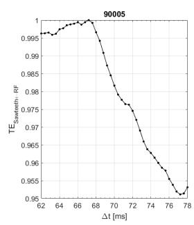
TE example for sawteeth pacing. The highest time interval for the coupling is  $(67 \pm 9)$ ms
