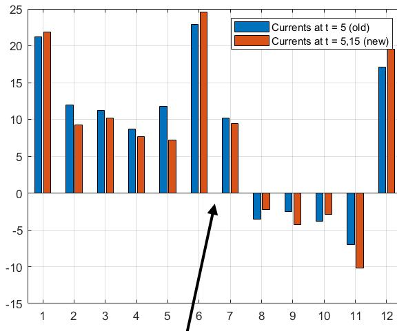
A tuning of CS/PF currents turns out to be necessary in order to fit plasma shape
