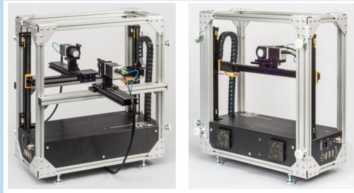
C.I.O. @ Leon (Mexico) experimental Set up Picometrix Two heads, with system lens of focal length of 13.5 cm , one emitter the other receiver, linked to the main seed laser by two 5 meter optical fibers.
