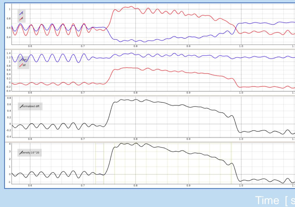
Measured signal of a typical plasma operation Argon #954 at  $I_e=10$ kA, equatorial line of view.
