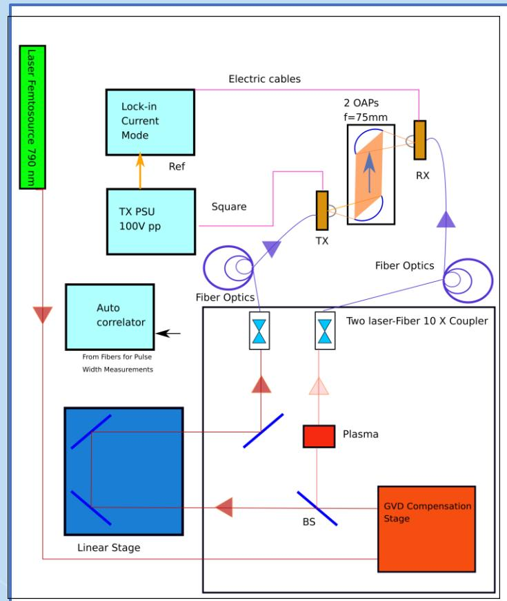
The IR laser radiation can be guided to the THz generation and detection devices by single mode optical fibers for considerable lengths (>10 m).
