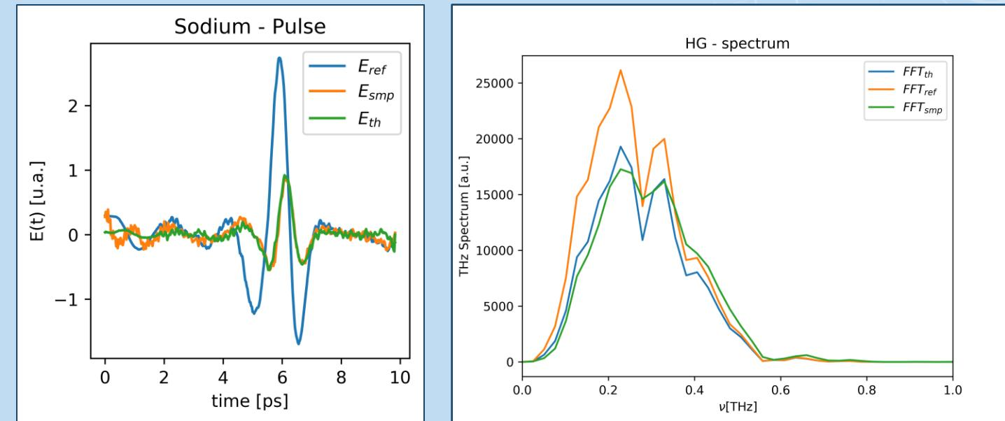
$$H(\omega, n_e, \nu_e) = \frac{S_{smp}(\omega)}{S_{ref}(\omega)} = \exp\left(i \frac{\omega L}{c} (1 - n(\omega, n_e, \nu_e))\right)$$
