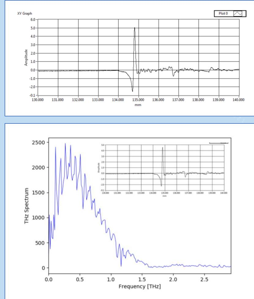
Example of measured pulse with electro optical sampling and relative Fourier Transform.
