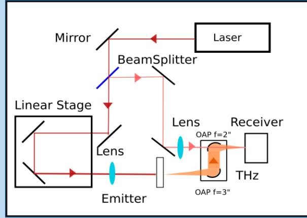
A Ti-Sapphire Mira 800 nm mode-locked laser. The device generates a 170 fs long pulse that is separated into two branches by a beamsplitter the pump branch where the THz pulse is generated and probe branch , where the THz pulse is detected. The linear stage introduces an optical path difference between the source and the detector.
