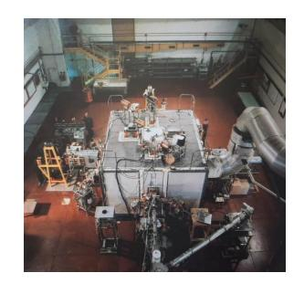
FTU machine (design & construction: 1982-1989, operation: 1990-2019), a medium-size tokamak with a circular poloidal cross section (major radius R0 = 0.935 m, minor radius a = 0.30 m), a metallic first wall, high plasma current (1.6 MA) and high magnetic field (8 T).
