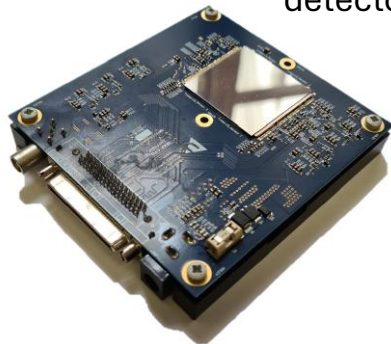
Timepix3 Silicon detector
