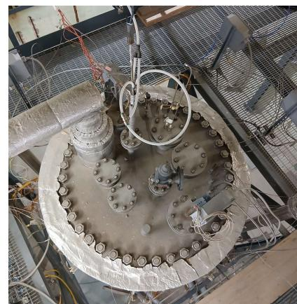
Tests of interactions between air and liquid lead are currently in progress, to study the oxygen diffusion inside the lead. Tests for the characterisation of different types of oxygen getters (Zr, Ti, Al) are also foreseen in the frame of the ANSELMUS Project.
