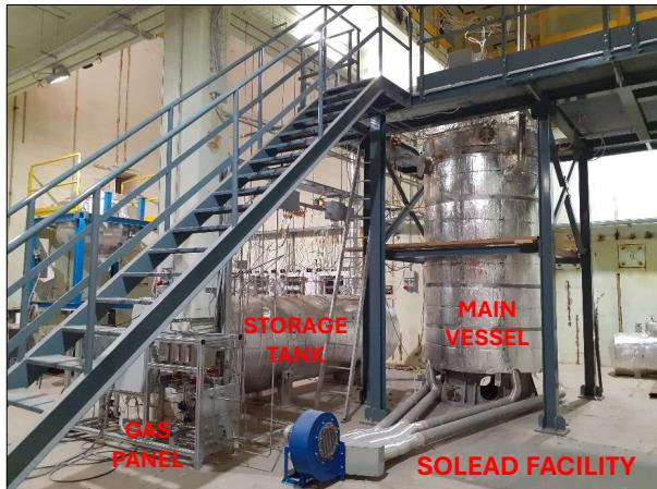
Under a collaboration agreement between **ENEA** and **newcleo**, the storage tank S100 was used for **corrosion tests**, in static conditions, on structural material specimens.
