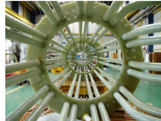
SC buslines with GFRP insulation
