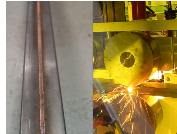
Laser welding (automatic)
