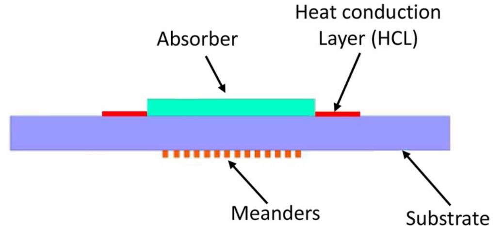
In case of mixed configuration (IPT and ITER) the absorber tickness can be customized.
