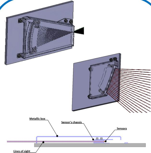
Different types of support are being considered to minimize the heat flux from the plasma and the divergence of the individual LoS, while still providing the best coverage of the plasma cross section
