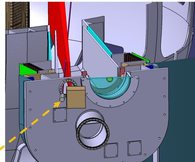
**Tangential GEM detector (included in the shielding box) and the high resolution SDD spectrometer updated layout (DTT Sector 8 port 3). Construction of an asymmetric GEM camera conceived to allow its positioning**
