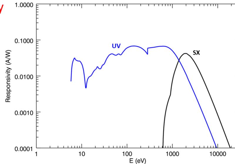
Calculated responsivity curves for the actual geometry of the detectors used on FTU; the calculation includes the Pt and Cr 5 nm contact layers, and the 6 mm Mylar filter for the SX detector.
