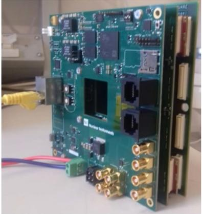
Fully assembled GEM detector with double FPGA acquisition board and front-end electronics (GEMINI chips).
